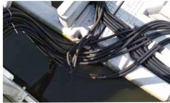
FIGURE 9.16 Biofouling on submerged connectors and cables
