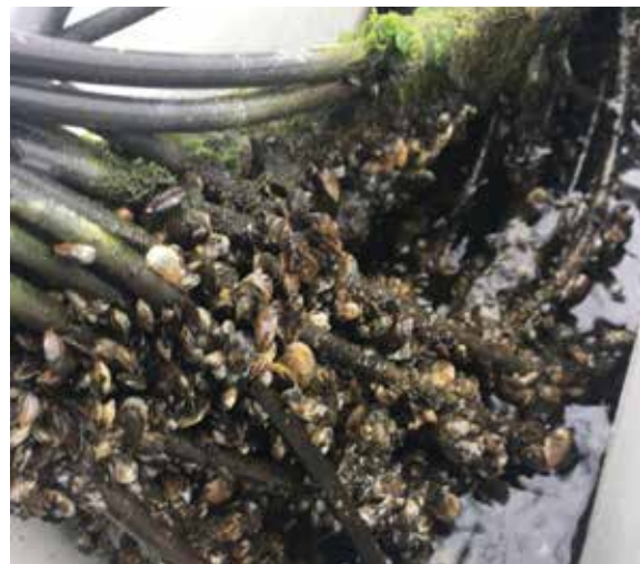
FIGURE 9.16 Biofouling on submerged connectors and cables
