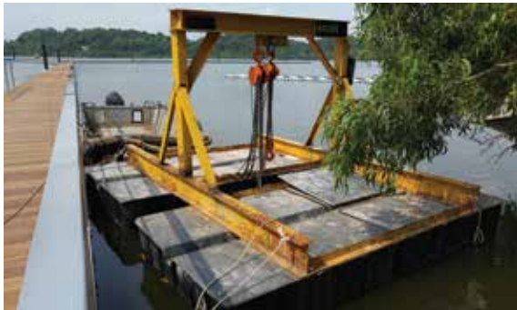
FIGURE 7.9 Barge used to lower concrete sinkers
