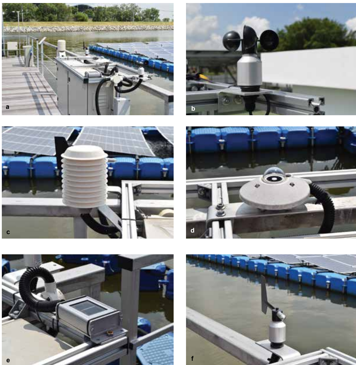
FIGURE 9.2 Meteorological station close to FPV system (a) and types of sensors: (b) wind speed sensor, (c) humidity sensor, (d) pyranometer, (e) Si-sensor, and (f) wind direction sensor
