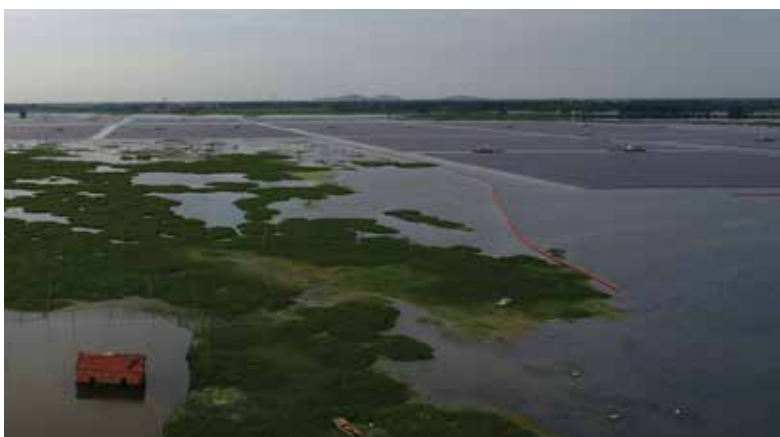
FIGURE 4.1. Coal mine subsidence area in Anhui Province, China, rehabilitated with Sungrow Guqiao 150 MWp FPV system. Left: after construction of FPV system; right: local people employed by Sungrow
