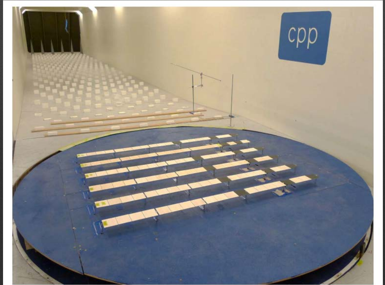
Figure 1: Wind tunnel model of the NEXTracker array section.
