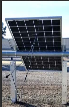
Testing rear tube effect at Center for Solar Excellence
