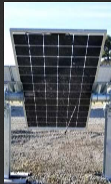
Testing rear tube effect at Center for Solar Excellence
